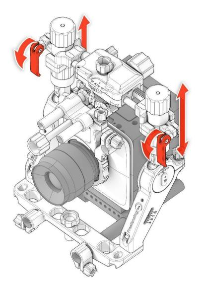
ADJUSTING SCREW (M3) from the locking cam for Y-shift (pay Special attention to the pressure of this screw, as it could loosen due to vibrations during transport).
