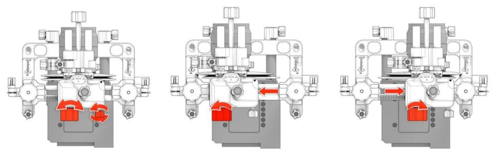
LOCKING SCREW for X-shifting
