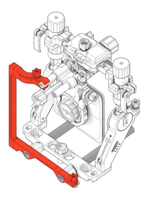
Use the cage with U shape included in the kit to fix the system and avoid vibrations. The system will suffer due to vibrations during transportation if the U-cage is not attached.
