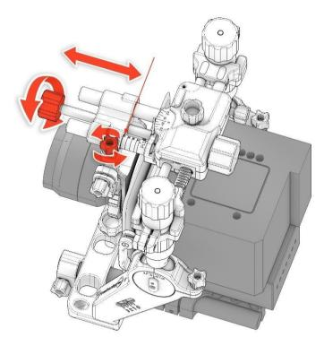
LOCKING SCREW for Zshift "collimation"
