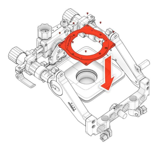
For SONY VENICE & RED DSMC2 when attaching the screws, the operator must always look at the "UP" side of the mount  $\rightarrow$  and see the position of the upward arrow.
