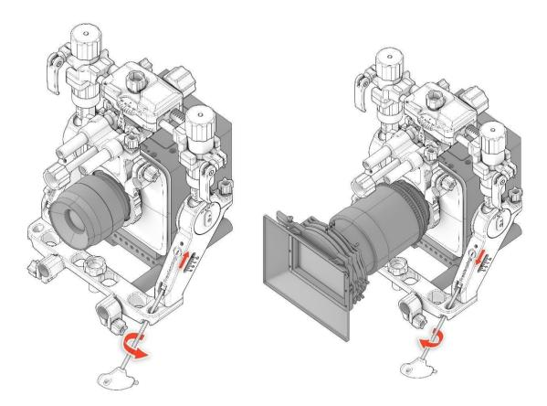
Adjustment: the counterbalance counteracts the gravity drop of the lens, allowing it to float, i.e., in neutral position in front of the sensor.
